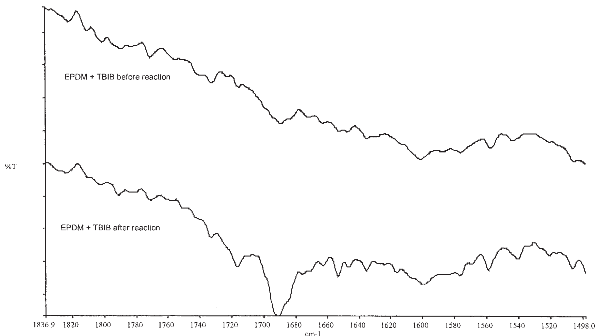
Figure 2 FT-IR ATR-spectra of TBIB + \alpha -MeS + EPDM before and after dynamic curing reaction: expansion of the carbonyl region.
